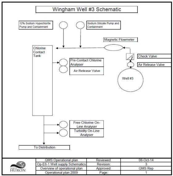
[Source: North Huron QMS Operational Plan, Revision 3, October 8, 2014] Note: This process flow diagram is for reference only, and represents a high level overview of the system as of October 2014.
